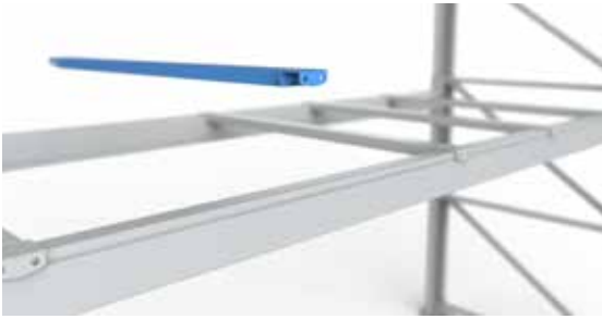
BEAMS FOR 4S AND 4C CROSSBEAMS
